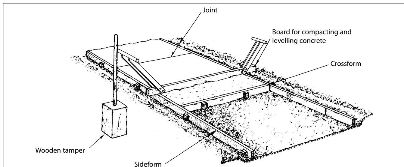
**The panel at the back has been completed, that in the middle has been laid and is being levelled and the base and formwork of the front panel have been prepared.**
