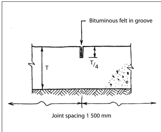
**Figure 2: Longitudinal section through road showing grooved joint**
