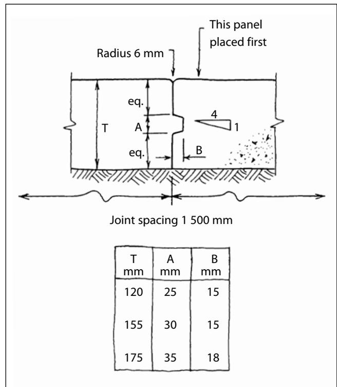
**Figure 3: Longitudinal section through road showing keyed joint**
